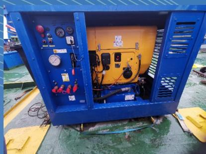
Hydraulic Power Supply HATZ with bio-degradable oil
