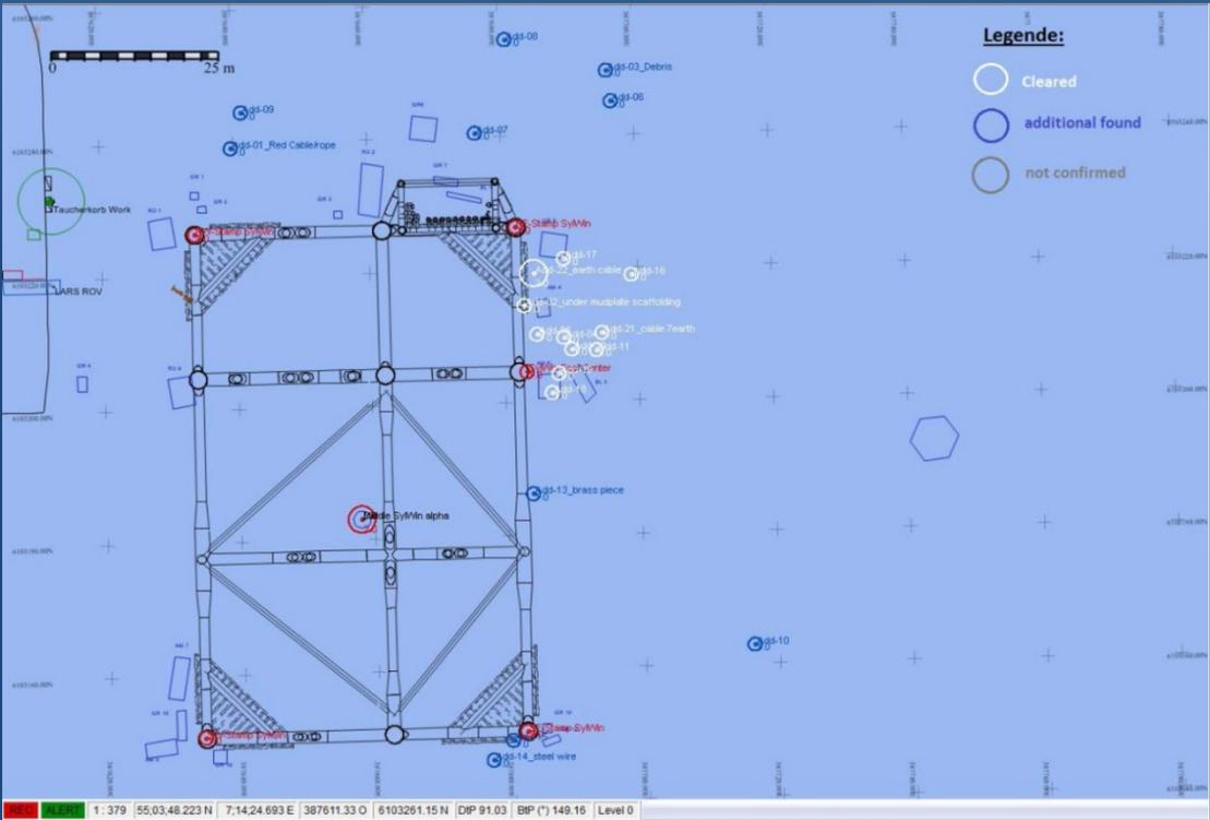
Logged target positions to support the divers and ROV's clearance tasks. After an initial survey additional targets identified can be added. The work progress can be monitored and documented. An as left survey of located targets is more simply and faster.
