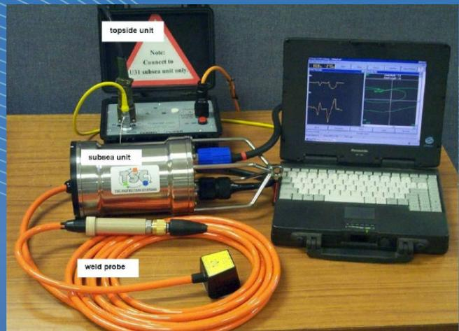
U31D Crack Micro Gauge System (with short test umbilical)
