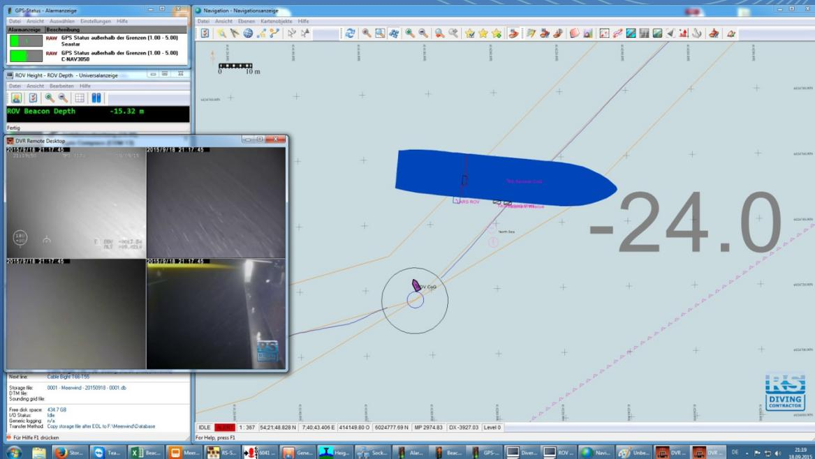
ROV Inspection tracked by QINSy showing the ROVs depth and position to navigate the ROV as close and as fast as possible to the job task.
