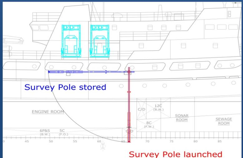
In lowered position, the flange of the pole is located approx. 0,5m under the keel of the vessel. Draught of the vessel is approx. 4,6m.
