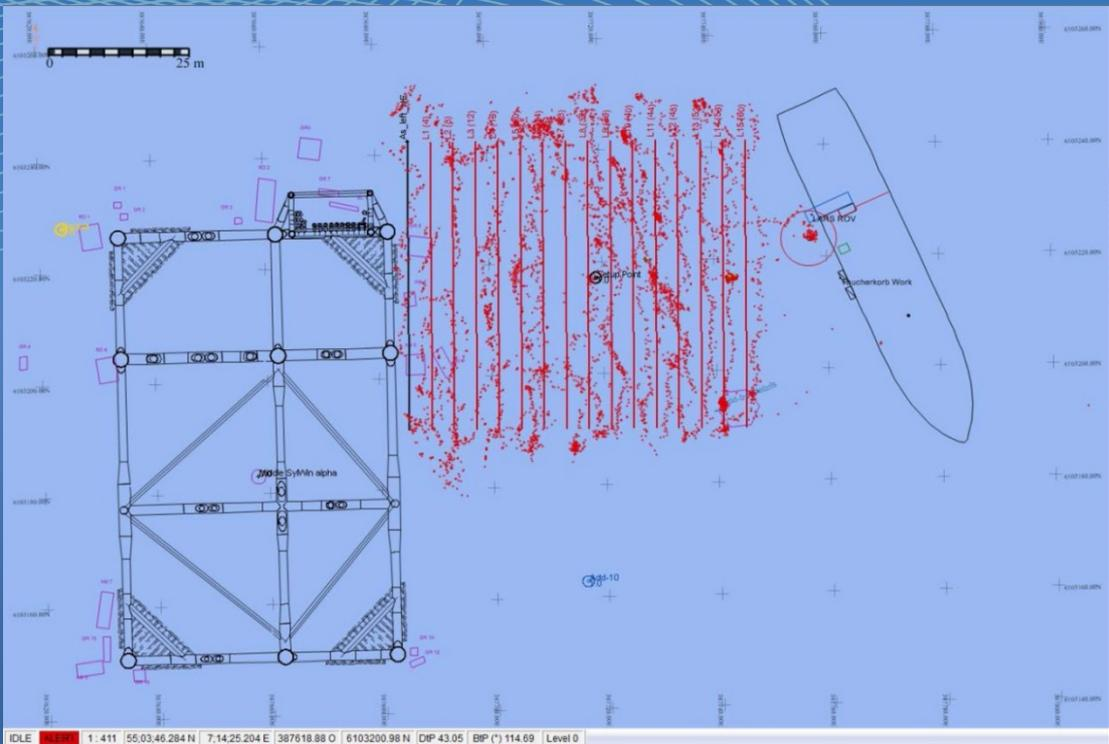
Logged positions of an ROV video inspection across survey lines to ensure a 100% coverage along the required survey area.
