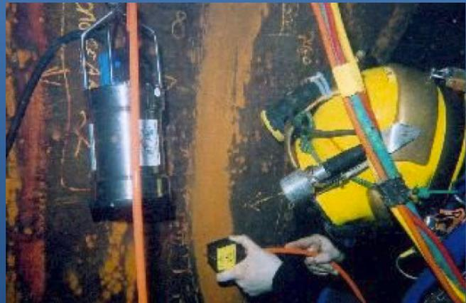
Diver uses the U31D Crack Micro Gauge System
